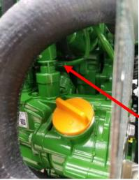
2) Locate fuel pressure sensor as shown below. It can be found at the end of the fuel rail closest to the fan.
