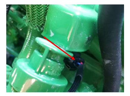
5) Connect the Stock Cummins connector to the Male Fuel Pressure Connector on the module harness.
