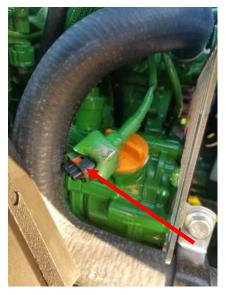
4) Plug Female Fuel Pressure Connector from module into fuel pressure sensor.
