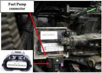
3) On the ADS module harness, the 6-pin female connector will now connect to the fuel pump.
