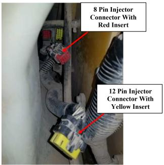
**4)** Plug the female injector connectors from the ADS harness into factory injector controller. Match the pin count and color to the factory controller.
