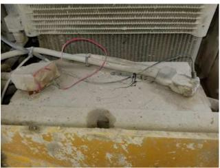
**7)** Mount the module with the connector on the bottom side, as to reduce the chance of moisture from getting into the module harness. Keep away from excessive heat and moving parts.
