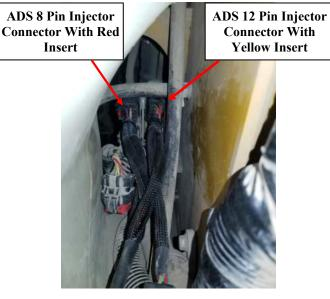
**5)** Plug the male ADS injector connectors into the factory female injector connectors. Again matching pin count and insert color.
