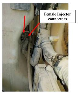
**3)** Unplug the two factory injector connectors shown by pulling back on the lock tab and depressing the release just forward of the lock. One connector will be a 12 pin with yellow insert, the other 8 pin with a red insert.
