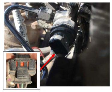
**Step 7)** )Insert the 3-Pin male connector from the module harness into fuel rail sensor. Make sure the connector latch is on the ramp side of the sensor.
