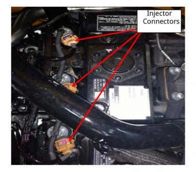
**Step 1)** Locate the stock Injector Connectors on top of the valve cover. There will be four in a row going to the injectors. These are two-pin female connectors.
