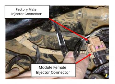
**Step 4)** On the module harness, now connect the female two pin connectors to the male injector connectors from the factory engine harness. Repeat the initial order by going from connectors D through A.
