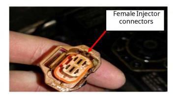
**Step 2)** Unplug all four of the stock injector connectors. Press and hold the release tab on the connectors and gently pull the connectors apart.
