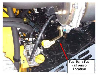
**Step 5)** Locate the fuel rail and the fuel rail sensor. The three pin male connector going to the sensor will be enclosed in a protective rubber weather shield.
