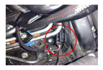
**Step 8)** Connect the Factory 3-Pin male connector from the engine harness to the female 3-Pin Connector on the Ag Diesel Solutions module harness.
