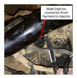
**Step 3)** On the module harness, the male connectors will connect to each individual injector. Injector connector D will connect to the injector closest to the flywheel. They will then connect in order with connector A ending on the injector closest to the fan/radiator.
