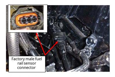
**Step 6)** Remove the factory three- pin male connector located on the engine harness from the rail sensor. Press and release the locking tab to disconnect.
