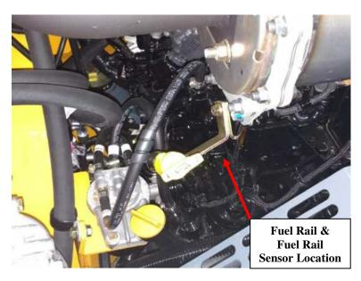
**6)** Remove the factory three- pin male connector located on the engine harness from the rail sensor. Press and release the locking tab to disconnect.
