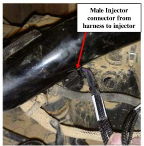
**4)** On the module harness, now connect the female two pin connectors to the male injector connectors from the factory engine harness. Repeat the initial order by going from connectors **D** through **A**.
