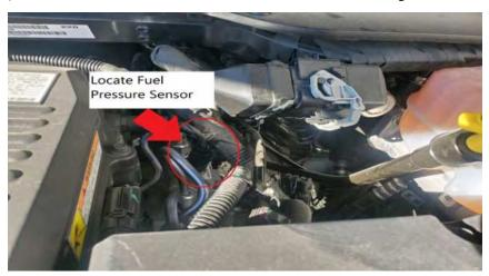
2) Disconnect the stock fuel pressure sensor connector. It is located at the center of the common fuel rail.
