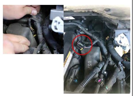
**3**) Connect the male connector from the module into the stock female fuel pressure sensor.
