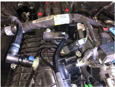
**5**) Disconnect the stock male T-MAP Sensor connector from the T-MAP Sensor.
