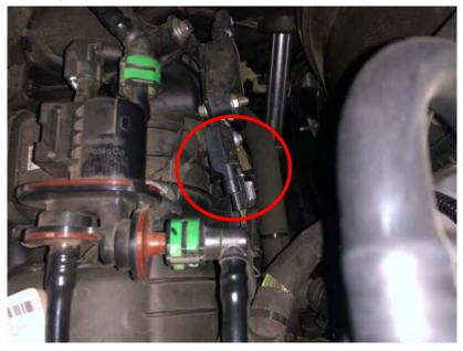
**4)** Utilize the portion of the Ag Diesel Solutions harness labeled MAP. Connect the male connector to the MAP Sensor. Then connect the ADS female connector to the stock male MAP Sensor connector.
