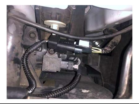
Remove the bypass plug from the Ag Diesel Solutions harness, and plug the harness into the module.
