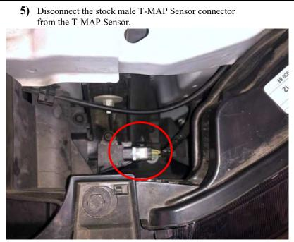
6) Utilize the portion of the Ag Diesel Solutions harness labeled T-MAP. Connect the male connector to the T-MAP Sensor. Then connect the female connector to the stock male T-MAP Sensor connector.
