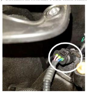
**4)** Utilize the portion of the Ag Diesel Solutions harness labeled MAP. Connect the male connector to the T-MAP Sensor. Then connect the ADS female connector to the stock male T-MAP Sensor connector.
