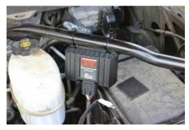
8) Connect module switch harness. Based on preference, the module switch can be secured in the engine compartment near the module or it can be routed into the cab. If mounting in the cab, route the Switch through the firewall and connect to the module harness.
