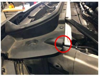
**4)** Disconnect the stock male MAP sensor connector by pulling back on locking tab and squeezing connector release tab.
