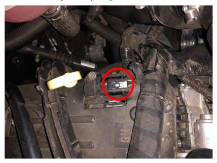
**5)** Utilize the portion of the Ag Diesel Solutions harness labeled MAP. Connect the male connector to the MAP Sensor. Then connect the ADS female connector to the stock male MAP Sensor connector.
