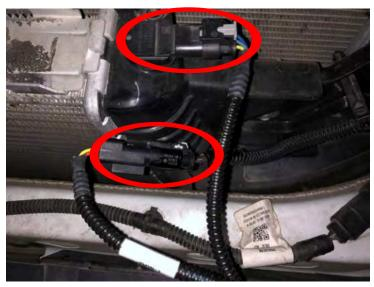
3) Reinstall dust cover with the harness exiting through the slot shown.
