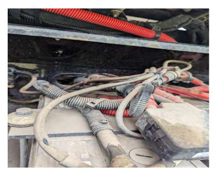
5) Hook up power and ground leads to batteries.
