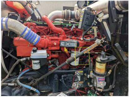
**2)** Disconnect the TOP ECM harness, as shown below. The correct harness is located to the right of the fuel filter. Note- You will have to unbolt bracket securing harness to ECM.
