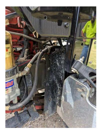
**4)** Locate any access hole through battery box and pull power and ground leads through to batteries.
